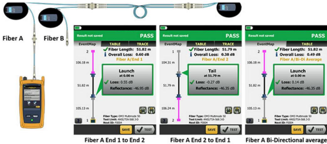
OptiFiber Pro's SmartLoop technology tests two fibers in one test while providing individual pass, fail and bi-directionally averaged results for each fiber link.
