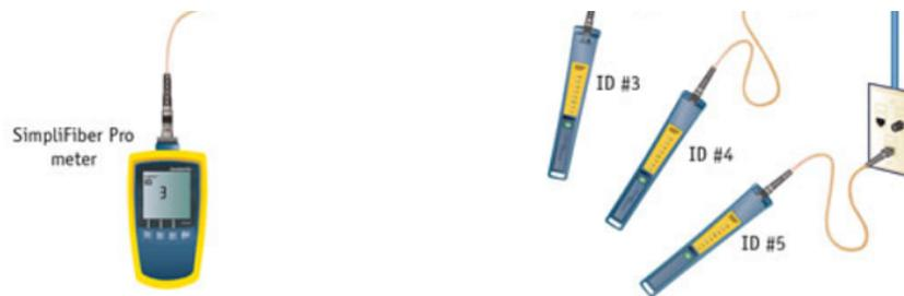
Figure 1 – Using FindFiber mode to locate fobers – patch panel to wall outlet
