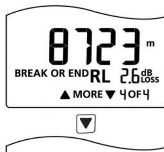
The result loss of the fiber (RL) is 2.6 dB.
