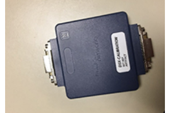
Figure 3 - One of the seventeen copper calibration artifacts as used in our service centers. Encased in plastic shell for protection.
